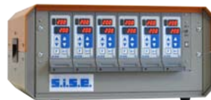
Coffret 8C6D -12 Zones Configuration COM
